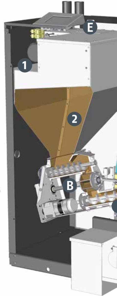
**1 Vacuum turbine for filling pellets**
